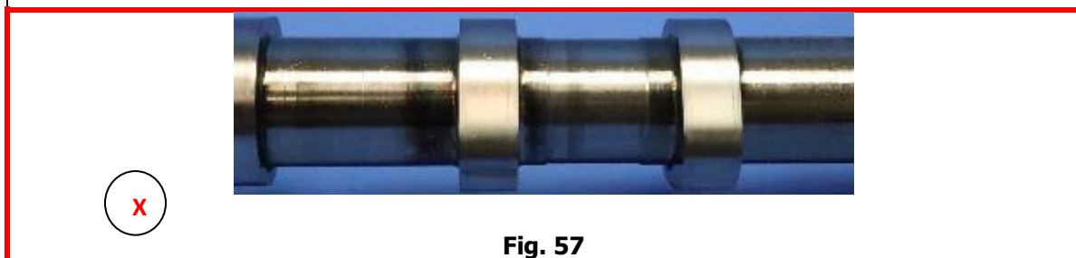
Examples of camshaft in not acceptable conditions
