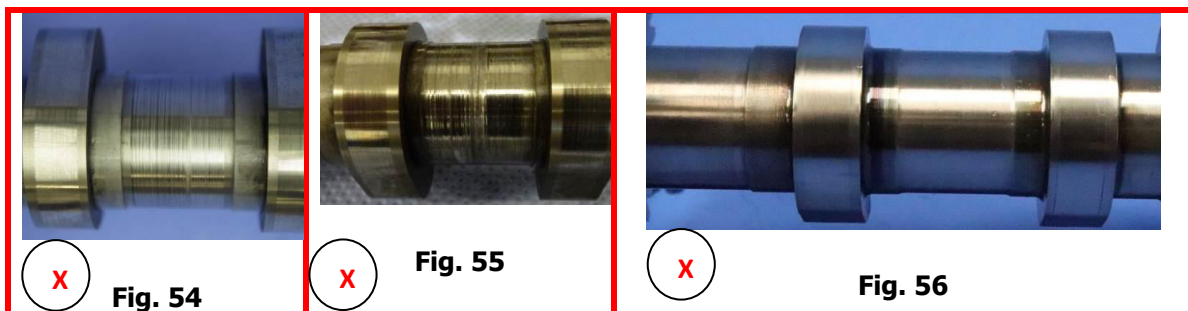
Examples of camshaft in not acceptable conditions
